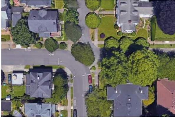
**Partial Diverters** – A partial barrier is a barrier that blocks one-half of a street. The barrier blocks the through movement in one direction.
